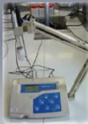
pH meter, acid / base titration, determination of the neutral points
