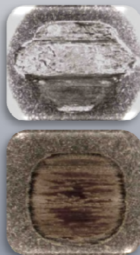
Additive influence on anti seizure performances of a grease
