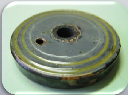
Coated sample after tribological test at 950°C
